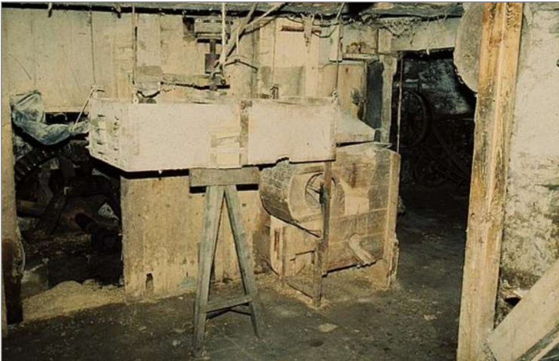
View of the gear cupboard with the Meal Sieve & Small Fanner still in place, prior to dismantling for restoration. © Mills Archive Trust: Jim Woodward-Nutt collection, 1983, image 10743 https://catalogue.millsarchive.org/benholm-harp
