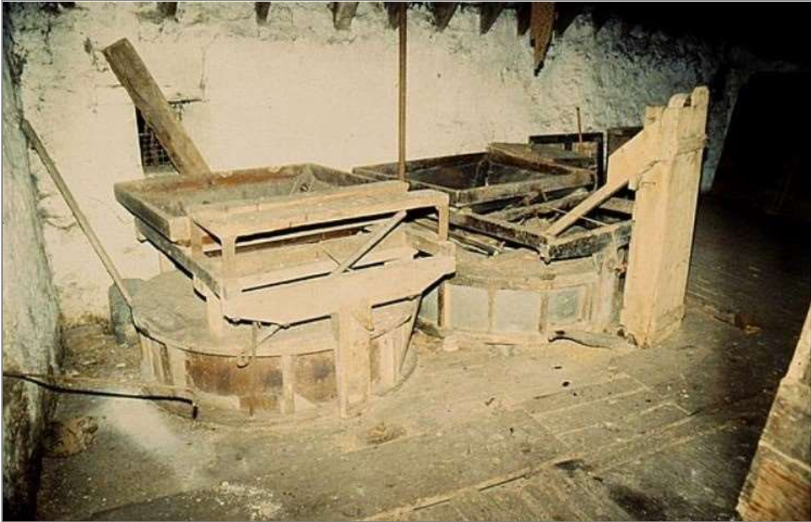
The millstones at the Mill of Benholm prior to any restoration works. © Mills Archive Trust: Jim Woodward-Nutt collection, 1983, image 10746 https://catalogue.millsarchive.org/benholm-st
