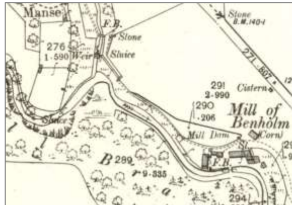
1901: 2 nd ed. OS shows the dam is no longer in place, either adapted by the miller or perhaps as a result of changes to the water courses or embankments. The dam has been replaced by a weir.
