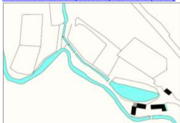
2023: there is effectively no change to the infrastructure excepting that the aqueduct (underground pipe) from the upper weir to the Castleburn is not functioning.
