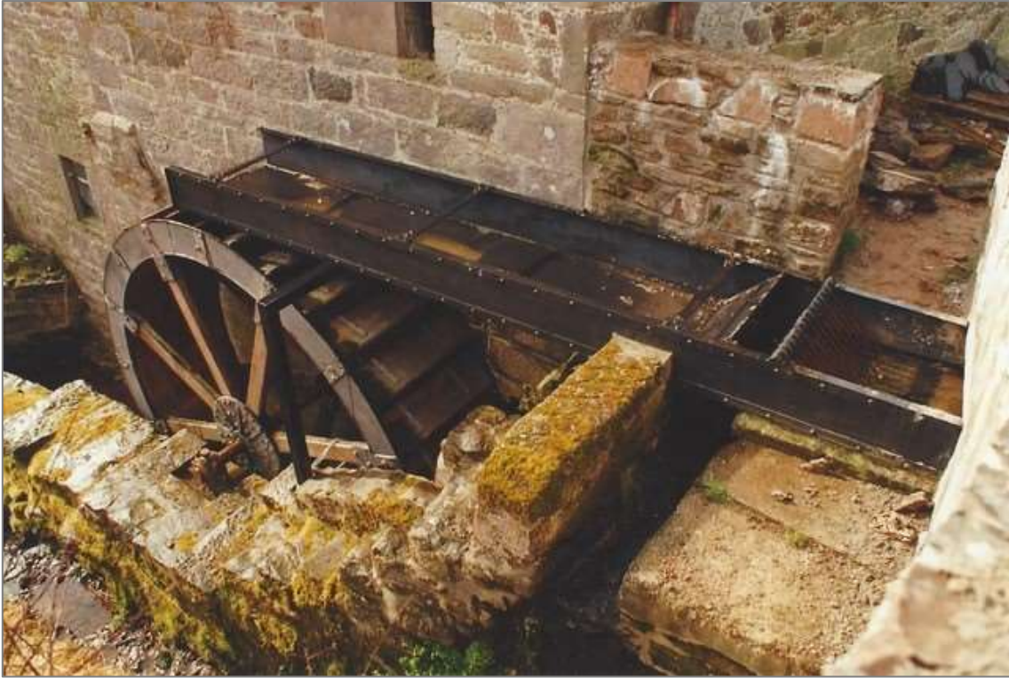
A view of the overshoot wheel at the Mill of Benholm, shortly after installation in 1992. Note the long trough known as a trowse which directs water from the mill pond via a culvert under the road to the top of the waterwheel (WE Ltd files).
