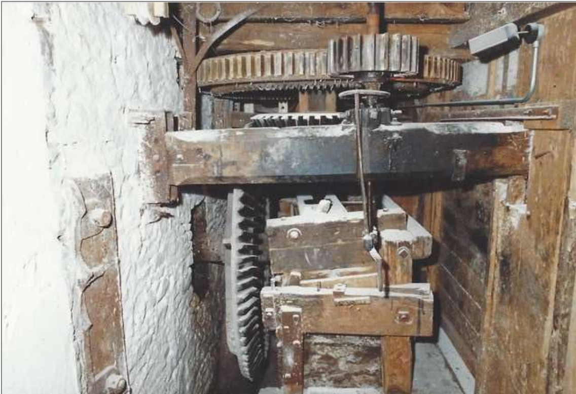
A view of the mill gearing at Barry Mill, Angus in 1992, note the large section timber, called the 'bridge trees', which supported the gearing for adjusting the milling stones (WE Ltd files).
