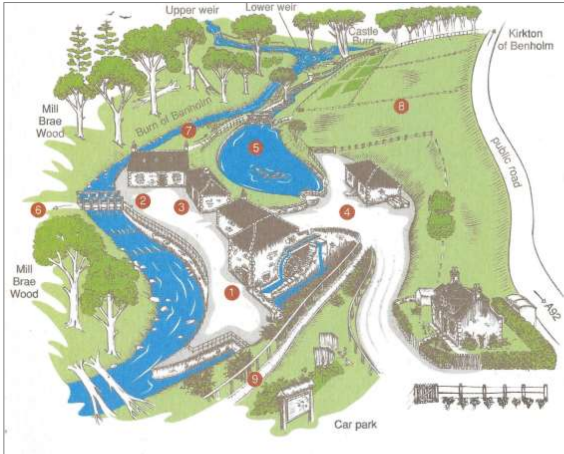
Mill of Benholm site drawing from Miller (1996) indicating the main buildings and features (refer section 1.4); note the later miller's cottage by the car park which is no longer part of the mill ownership. © Aberdeenshire Council.
