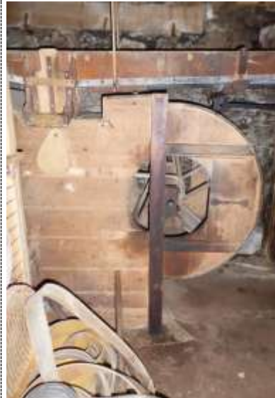
The Shaker , a long sieve, above the Large Fanner , note the internal paddles which create an air flow from the fanner.
