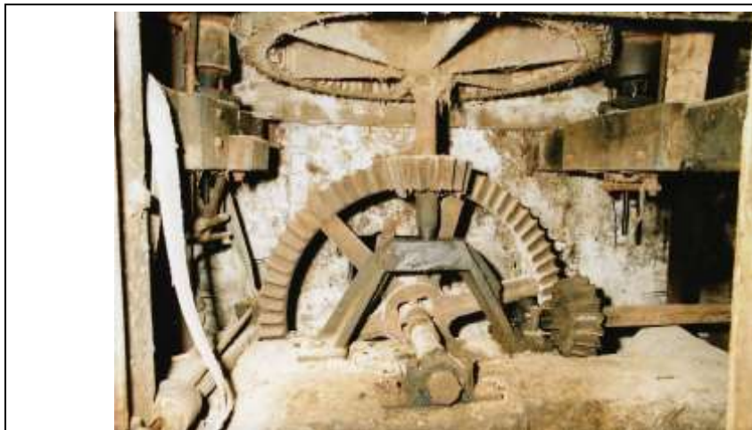
WE Ltd image (likely early 1991) before restoration works. Note the vertical Pit Wheel and the horizontal Great Spur Wheel above.
