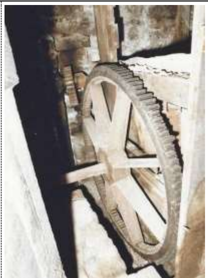
The Auxiliary Spur Wheel before restoration, note the worn and damaged wooden teeth (WE Ltd image).
