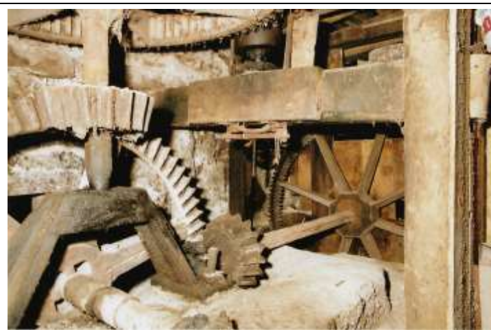
WE Ltd image (likely early 1991) before restoration works. Note the vertical Pit Wheel on the left and the vertical Auxiliary Spur Wheel on the right.
