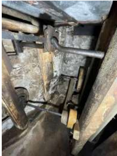
General view of crank shaft, pulleys and drive belts for the Shaker .
