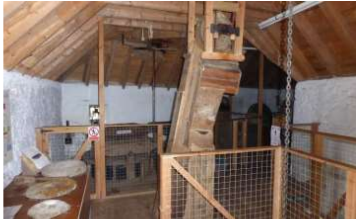
General view in 2023 looking east toward the Shelling & Grinding Stones with Bag Hoist and Bucket Elevator in the foreground.
