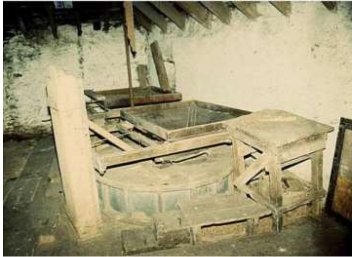
View of milling stones with the Grinding Stones in the foreground prior to adaptation. Note the earlier wooden steps for access to hopper not retained during restoration. © Mills Archive Trust: Jim Woodward-Nutt, 1983, collection image 10747: https://catalogue.millsarchive.org/benholm-st2
