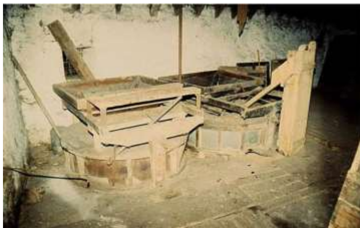
View of the millstones within their tuns and hoppers in place prior to restoration. © Mills Archive Trust: Jim Woodward-Nutt, 1983, image 10746: https://catalogue.millsarchive.org/benholm-st
